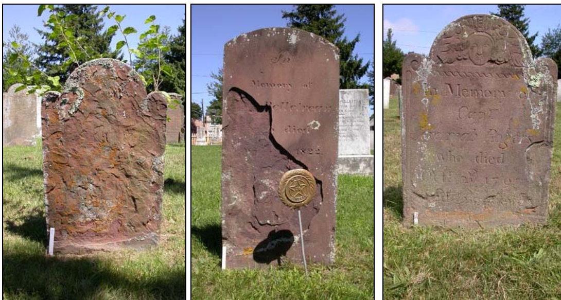
Blind delamination in Sandstone. Gone (left), Going (middle), Will go if hit (right)
